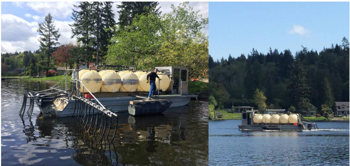
Figure 3. Chemical distribution system for April 2019 alum treatment
